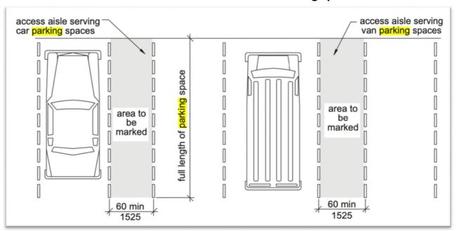
Parking Space Aisles [figure to be replaced with 5' access aisle drawing]
